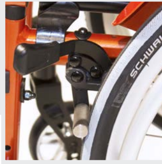
Unique brake with extremely low actuation force
