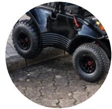
Obstacle climbing ability up to 110 mm
