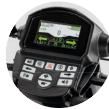
LCD colour display with illuminated keypad
